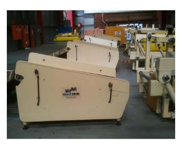
**Custom Built LC-Checkweighers for checking bundles of roof Insulation**
