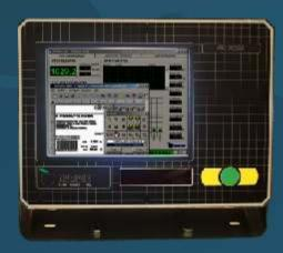
The 8" touch screen, applicable on the entire HSC350 model range, is provided with Wireless or Bluetooth connection and external infrared keyboard with trackball; with the execution of Windows™ tasks, it allows an easy integration of different printers and a client-side connection with plant database.
