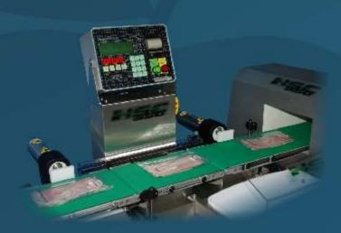
Checkweigher & Metal-detector - Serie M-L Multi or Mono frequency
